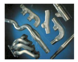
Figure 1. Components manufactured by THF
