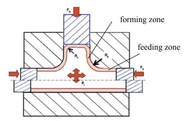
Figure 2. Feed and forming zones in THF process
