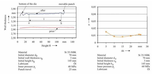
Figure 4. Wall thickness distribution prior and after upsetting
