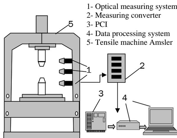
Figure 1. System for determining of flow curve
