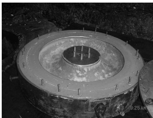
Figure 3. Die ready for underwater explosion
