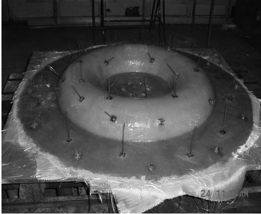
Figure 1. The master coated with epoxy resin reinforced with fiber-glass
