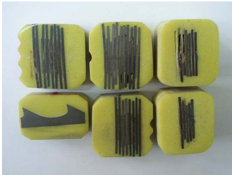
Fig. 1 Test samples prepared for the microstructural and microhardness testing
