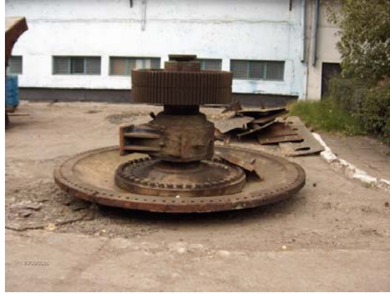
Figure 7. Front view of the cylinder after disassembly
