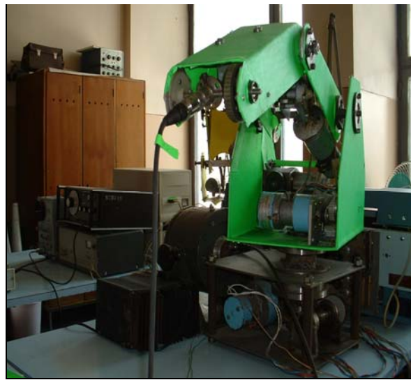
Figure 1. Experimental stand of the arm type robot to validate the mathematical model
