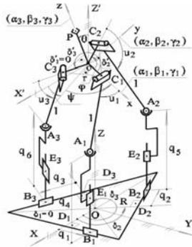
Figure 3. Kinematic scheme of the 3-PPSR mini-manipulator
