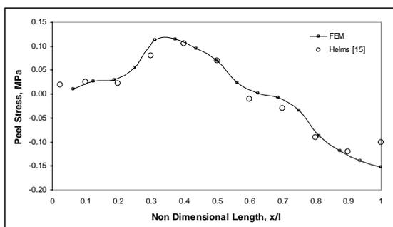
Figure 2: Adhesive peel stress
