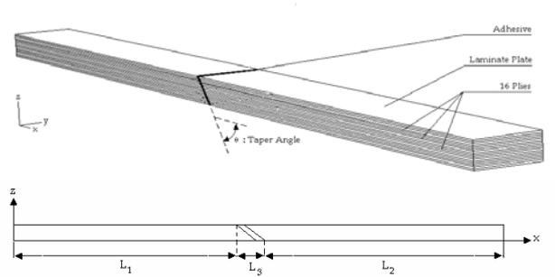
Figure 1: Geometric Configuration of taper-taper joint for laminated
