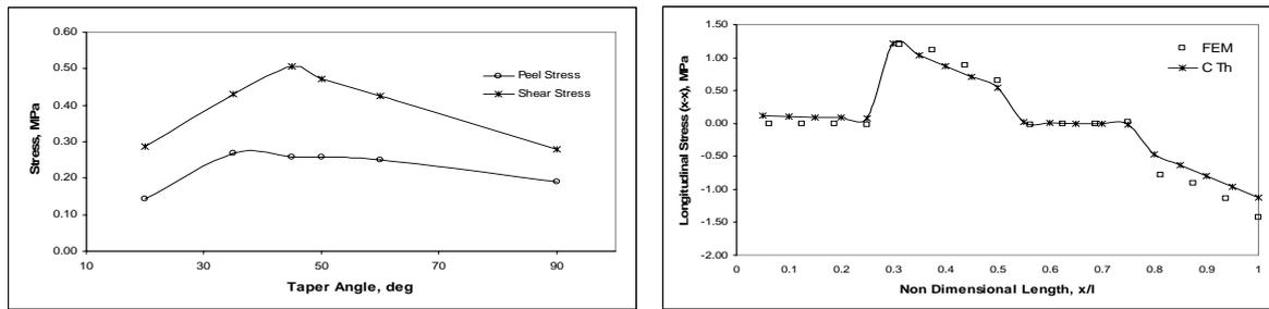
Figure 4: Peel and shear stress vs. taper angle Figure 5: Longitudinal stress distribution in adherends
