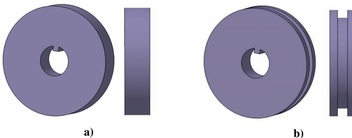
Figure 1. Sample for chip-chunk test: a) before the test, b) after the test
