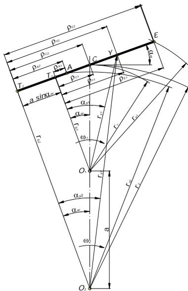
Figure 2. Radii of curves at specific points at contact lines for internal mesh
