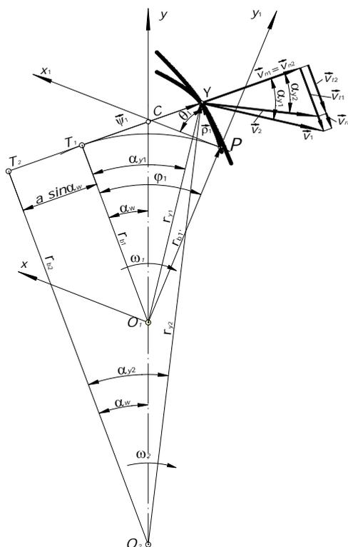
Figure 1. Internal mesh for a couple of gears
