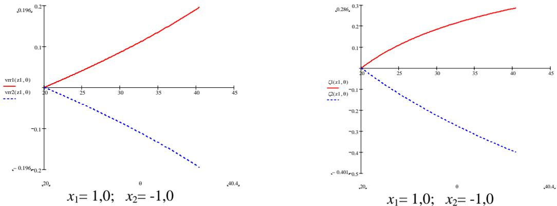
Figure 4. Profile deviation ratios' influence on sliding velocity and specific sliding at mesh interval  $\overline{AE}$
