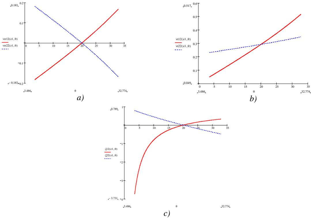
Figure 3. Variability of the sliding velocity (a), relative velocity (b) and specific sliding (c) at mesh interval  $\overline{AE}$
