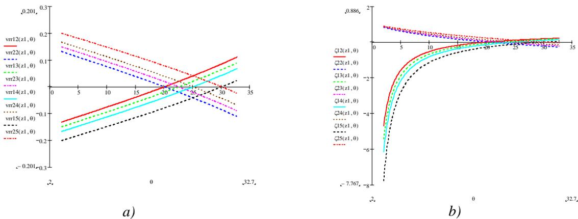
Figure 5. Influence of the angle of teeth's contact curve on sliding velocity (a) and specific sliding (b)
