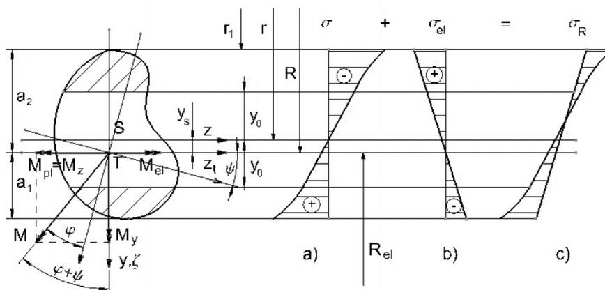
Figure 1. The elasto-plastic bending process: a) loading, b) unloading, c) resulting stress state.
