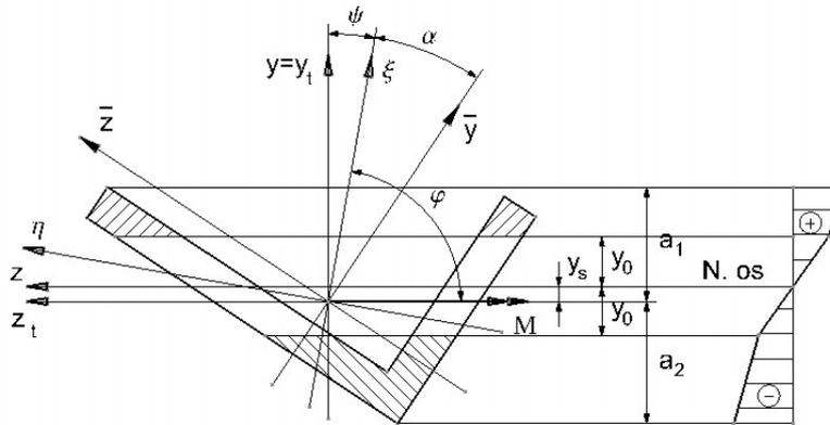
Figure 2. Loading state of cross section L 15x10x1.5.
