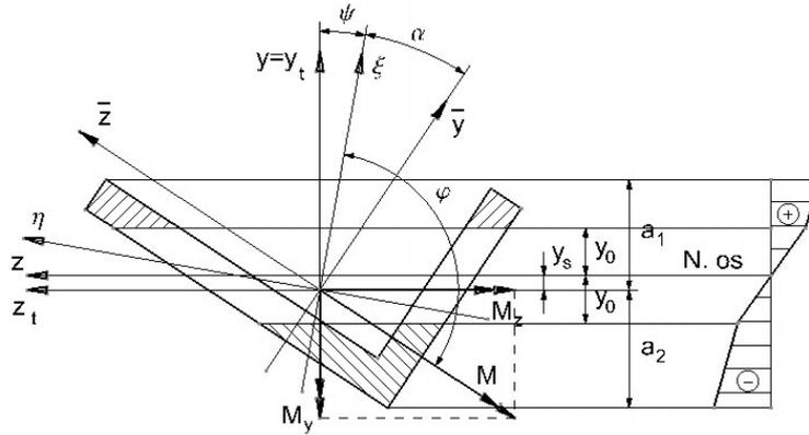
Figure 3. Loading state of cross section L 15x10x1.5.
