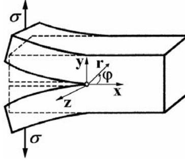
Figure 1. Illustration of mode I
