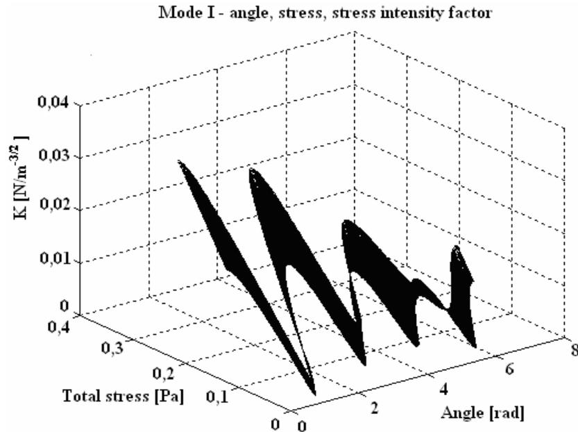
*Figure 2. PZT-4 ceramic's simulation results - total stress and stress intensity factor for  $r = 0,2a$  to  $3a$*
