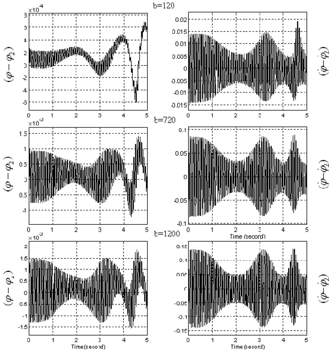
Figure 4. Graphically presented results for different values of dynamic absorber coefficient
