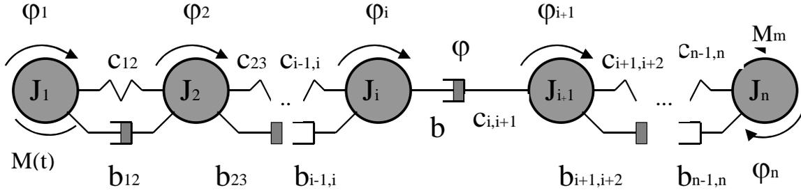
Figure 1. Dynamic model of a system with  $n$ -masses
