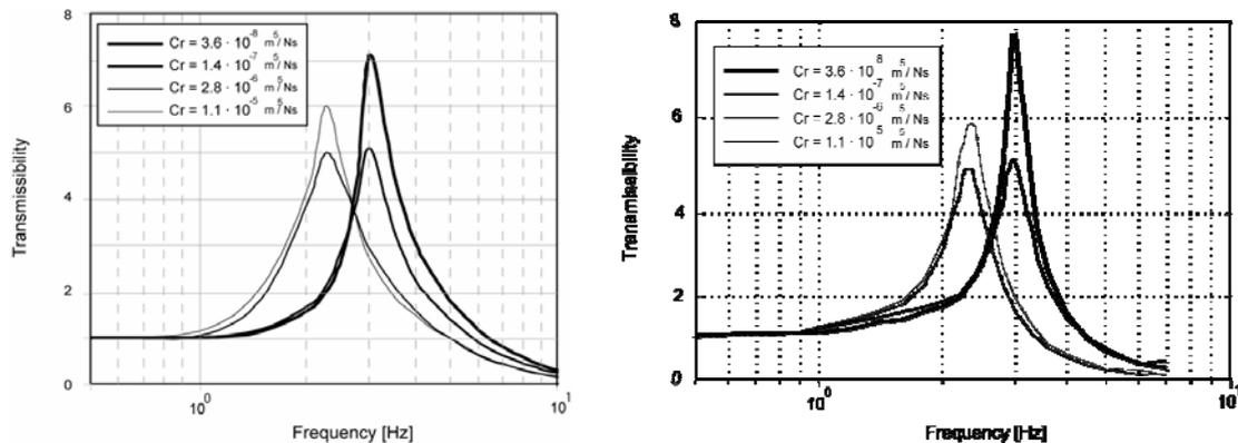
Figure 3. Modulus of the transmissibility function for the nonlinear model (left), and the experimental tests (right).
