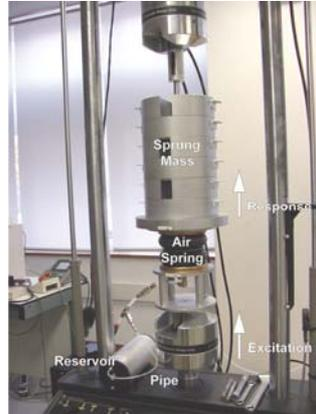
Figure 2. Experimental assembly for the pneumatic suspension.
