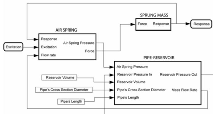
Figure 1. Analytical model of the pneumatic suspension in Simulink environment.
