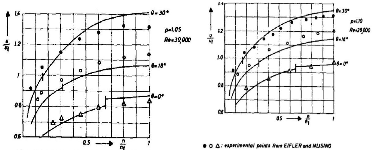
Fig. 3. Calculated and experimental velocity distributions
