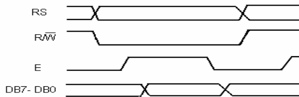
Figure - 2. Timing diagram of writing data to LCD
