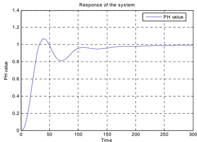
Figure 6. Response of the system on step input
