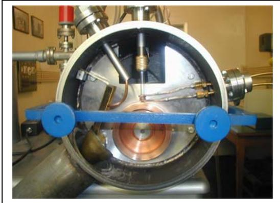
Figure 1. part of the device for production of amorphous strips
