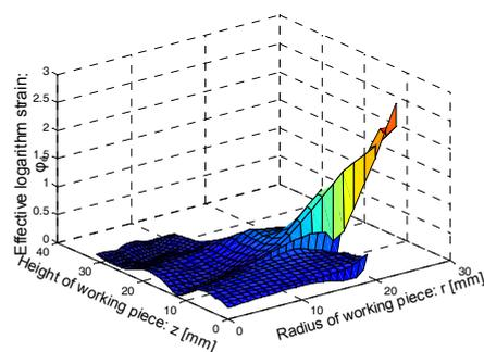
Figure 3. Effective logarithm strain:  $\phi_e$
