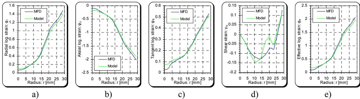
Figure 4. Comparing deformation parameters obtained by PDM and regression analysis i cross-section of wreath plane of working-piece: a) Radial logarithm strain; b) Aksial logarithm strain; c) Tangent logarithm strain; d) Shear strain; e) Effective logarithm strain
