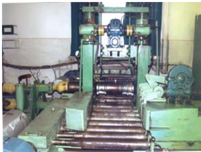
Figure 4. The assemblies of the mill stand with the attendance equipments
