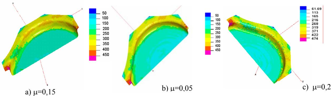
Figure 5. Stress distribution after finishing deep drawing process
