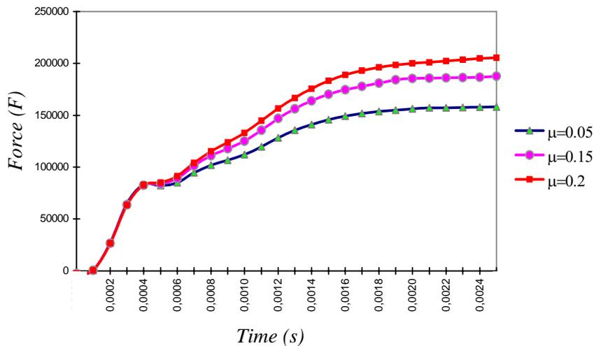
Figure 4. Diagram of distribution contact force blank – die during deep – drawing process process for different friction coefficient
