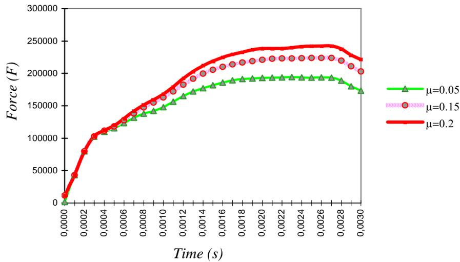
Figure 3. Diagram of distribution contact force blank- punch during deep drawing process for different friction coefficient
