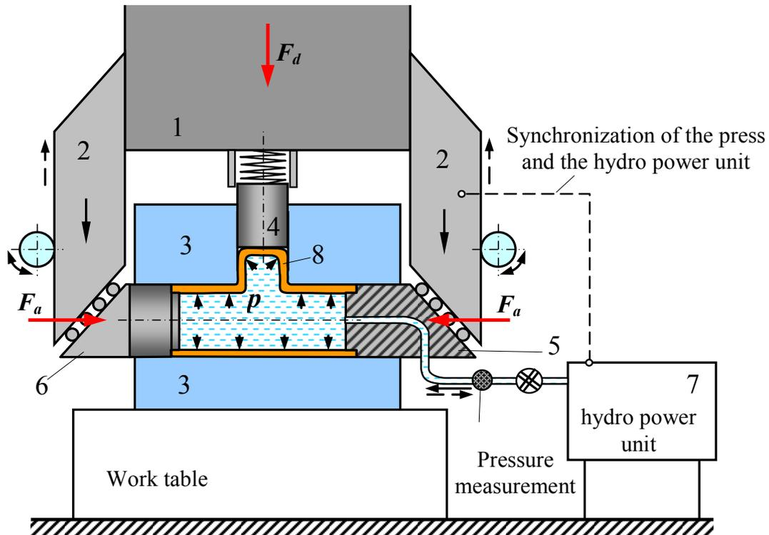
1- Punch 2- Built in additional sliders. 3- Die. 4- Counter punch. 5- Multiplication of pressure (punch of axial hollow for the intake of fluids). 6- Piston – axial punch. 7- Hydro power unit with all needed elements (measuring, safety, regulation). 8- Forming of tubes under pressure  $p$ .
