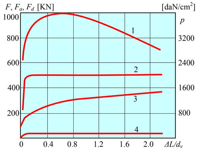
Figure 4. The change of force  $F_i$  in the hydroforming process of  $T$  shape tube,  $\phi$  25 mm from steel:
