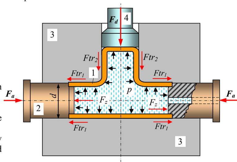
Figure 3. Schema of hydroforming process T-shape and forces
