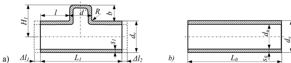
Figure 1. Tube workpiece (a) and initial piece (b)
