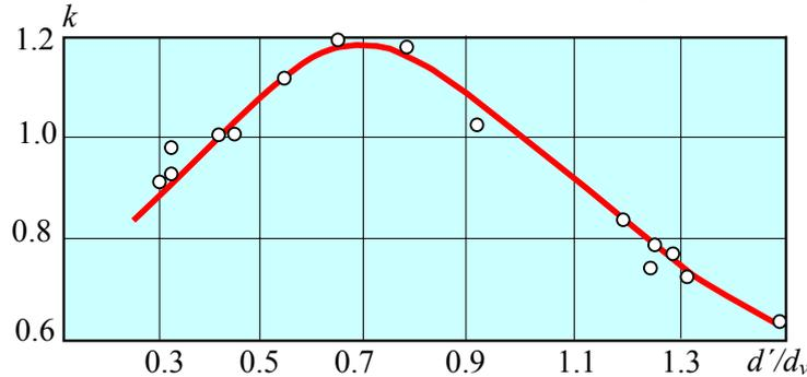
Figure 2. Correction coefficient depends on the relation between the diameter  $k - f(d'/d_v)$
