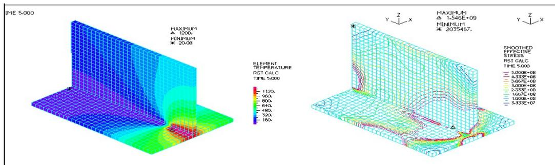
Picture 1. 3D model, Presentation of distribution of temperatures and stresses
