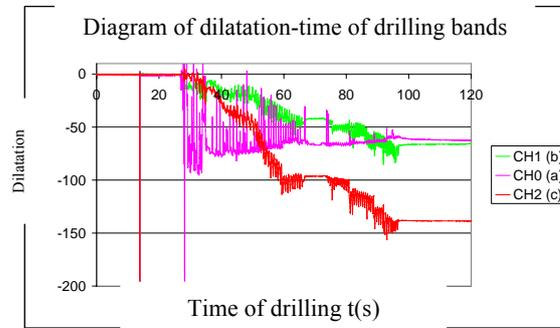
Picture 2. Diagram of measuring of dilatations during drilling of sample through rosette
