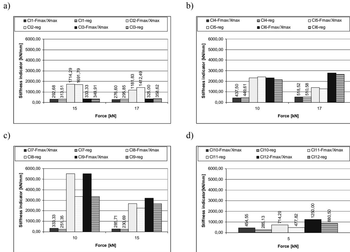
Figure 3. Comparison of stiffness indicators' values UBF-112 N machine tool
