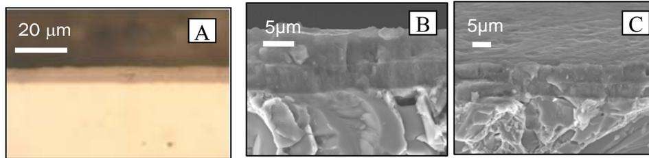
Figure 4. Optical microscopy (A) and SEM fracture cross-sections of TiAlN coating (B, C).
