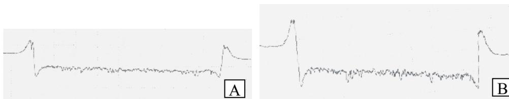
Figure 1. Crater shape after a GDS experiment performed for 100 s (A) and 150 s (B) on TiAlN deposited on AISI D2.
