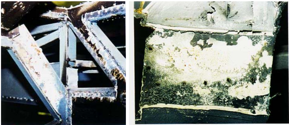
Figure 1. The examples of corrosion occurring on the parts of vehicle directly contacting with outer
