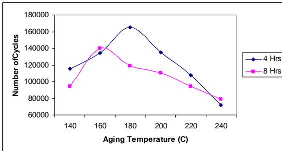
Figure 1. Effect of aging temperature and time on fatigue fracture properties of 6063 AA; no hydrogenation
