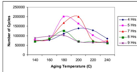
Figure 2. Effect of aging temperature and time on fatigue fracture properties of 6063 AA; 1.5 hours of hydrogenation
