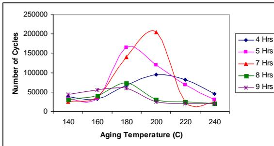
Figure 3. Effect of aging temperature and time on fatigue fracture properties of 6063 AA; 3 hours of hydrogenation
