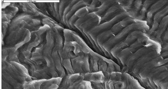
Figure 5. Micrograph of fatigue surface of sample aged for 4 hours at 160°C and hydrogenated for 3 hours
