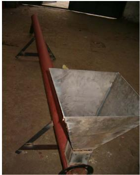
*Figure 2. Experimental installation for adding covering and thermoisolating powder in tundish*
