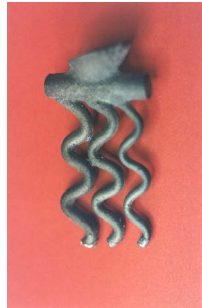
Figure 3. D pattern cast from Wiroloy alloy, with the diameters of the branches of 2.5, 2 and 1.5 mm
