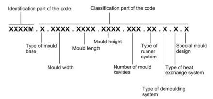
Figure 3. Mould classification code
