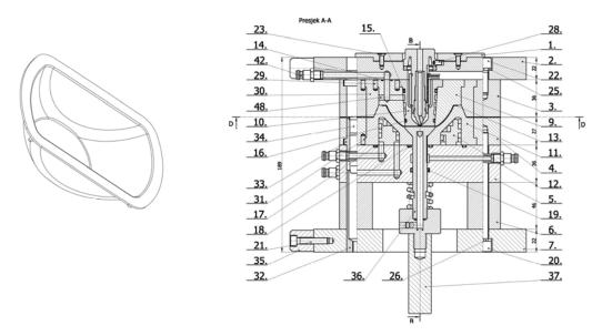
*Figure 4. Example of thermoplastic moulded part and the respective injection mould* [7]
