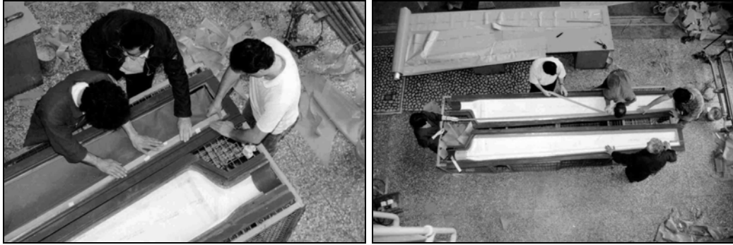
Figure 3. Assembly of the mold and work on blade halves
