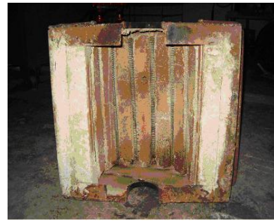
Figure 2. The electric furnace having four curled spirals
