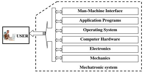
Figure 1. Components of a mechatronic system.
