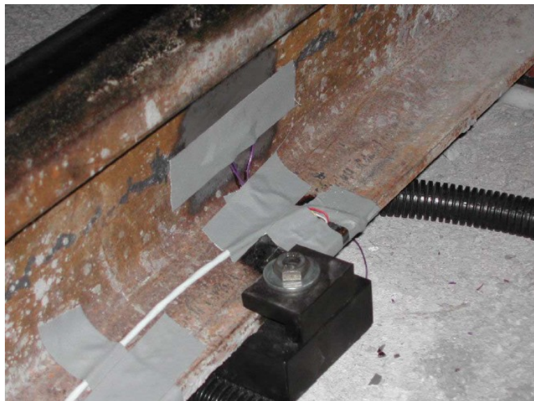
Figure 1. Accelerometer placed at the bottom of the rail and strain gauges sensor placed in the rail web.
