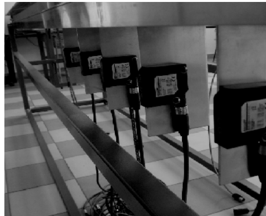
Figure 4. View of row of laser heads at left rail
