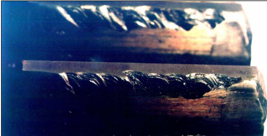
Figure 2. Working surfaces of the teeth hardfaced with additional material UTP 670 after 98 \cdot 10^6 cycles
