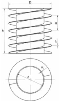
Fig. 1. Experimental helicoidal shell on cylindrical shell model
