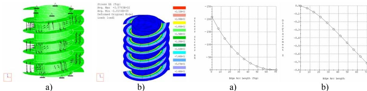
Fig. 6. FEA for model and helicoidal shell thickness  $h_h = 3.6$  mm: a) meshed model with loads and constraints, b) distribution of the radial stress
