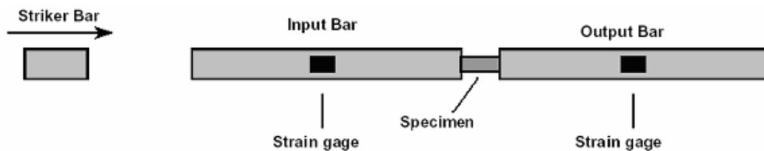
*Figure 1. Schematic of Split Hopkinson Pressure Bar*
