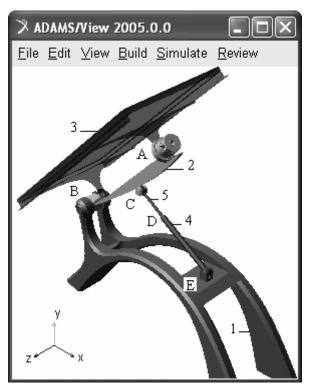
Figure 1. The virtual prototype of the PV system.
