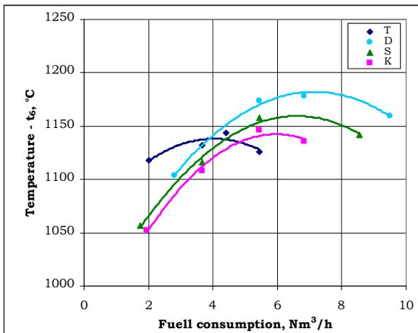
Figure 8. Average temperature of the combustion chamber depending on the fuel consumption and geometry changes; geometry: code 41, 42, 43, 44
