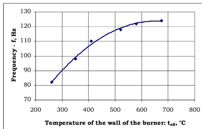
Figure 2. Influence of the wall temperature on the process frequency; geometry: code 41, fuel consumption:  $5,15 \text{ Nm}^3/\text{h}$  gas, resonant pipe: free end
