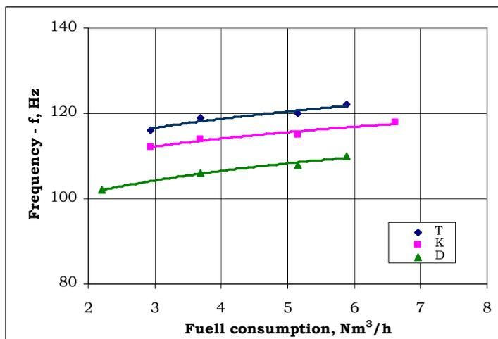
Figure 4. Frequency of the pulsating combustion process in a water-cooled burner; geometry: code 21, 22 and 24, (MK~); resonant pipe – position "d" inside the exhaust duct
