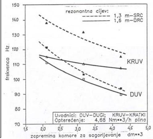
Figure 5. Change of the pulsation frequency depending on the geometry of the air-cooled burner; fuel consumption:  $4,68 \text{ Nm}^3/\text{h}$
