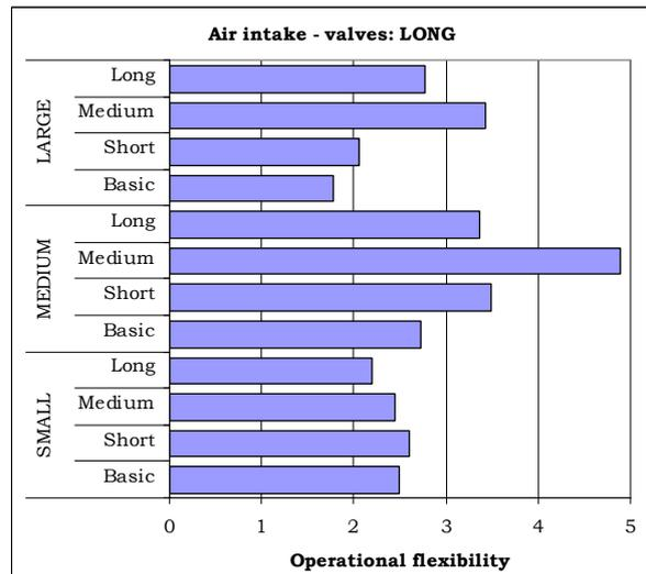
Figure 9. Operational flexibility of the water-cooled burner with long air intake-valves
