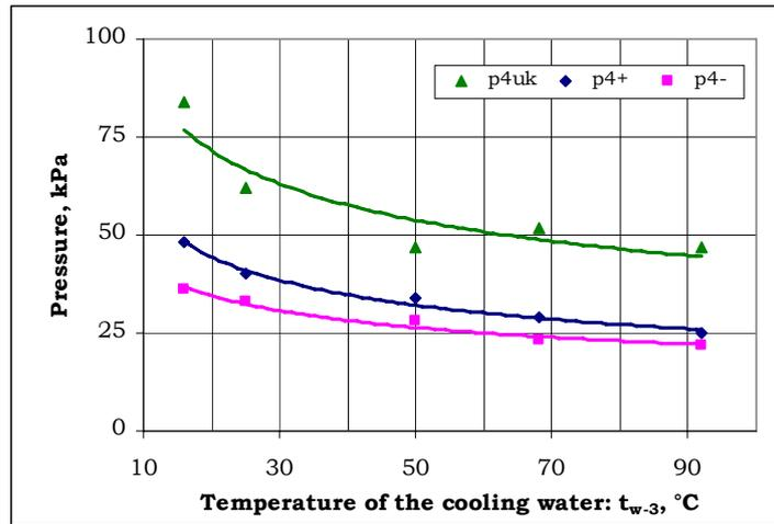
Figure 3. Changes of the pressure inside the combustion chamber depending on the cooling intensity:  $p_{4uk}$  – total change,  $p_4^+$  – positive,  $p_4^-$  – negative; geometry: code 44, fuel consumption:  $4,42 \text{ Nm}^3/\text{h}$ , resonant pipe: free end
