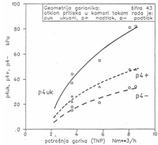
Figure 7. Form of the pulsating pressure inside the combustion chamber and the oscillating intensity changes when varying burner load (air-cooled burner); geometry: code 43, burner off limits 1,74 ÷ 8,6 Nm<sup>3</sup>/h
