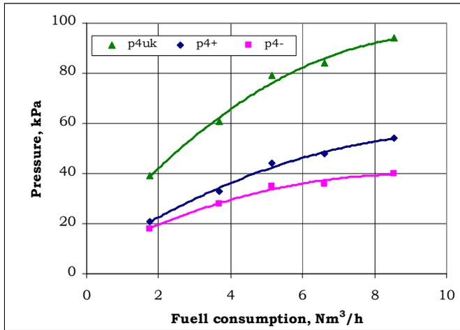
Figure 6. Form of the pulsating pressure inside the combustion chamber and the oscillating intensity changes when varying burner load (water-cooled burner); geometry: code 43, burner off limits 1,75 and 8,55 Nm<sup>3</sup>/h
