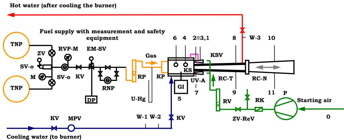
Figure 1. Water-cooled pulse combustion burner; parts of the test rig with measurement positions
