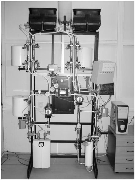
Figure 1. A photograph of the laboratory heating system
