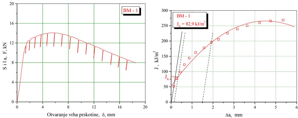
Figure 1. Diagrams  $F - \delta$  and  $J - \Delta a$  for the specimen with a notch in BM [1]
