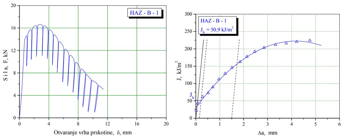
Figure 3. Diagrams  $F - \delta$  and  $J - \Delta a$  for the specimen with a notch in WM - Tehnology B [1]
