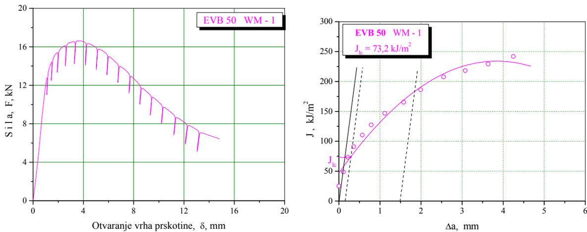
Figure 2. Diagrams  $F - \delta$  and  $J - \Delta a$  for the specimen with a notch in WM - EVB 50 [1]
