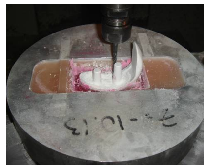
Figures 3, 4 and 5. Different steps in prostheses machining
