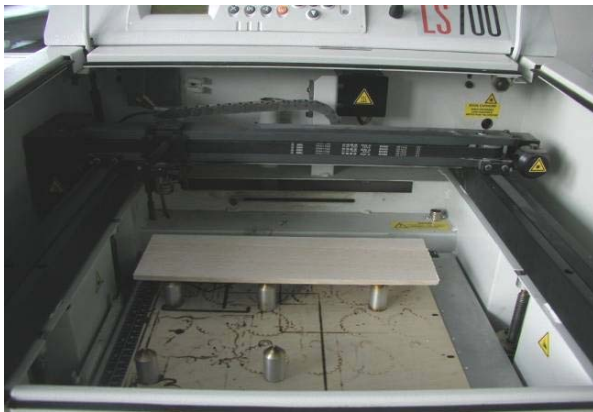
Figure 2. Placement of balsa board on a Laser LS700 30W
