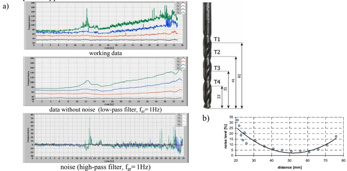
Figure 5. a) measured temperature with respect to time ( $E=1$ ) for some points on tool axis; b) relative noises level of temperature value measured at specified point of tool axis as a function of points distance from top of tool.
