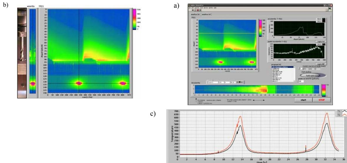
Figure 3. a) main window of application for thermovision images sequence analysis; b) view in visible range and IR range of driller top and linear temperature distribution of driller axis with respect to time; c) reflector temperature with respect to time  $T_r=f(t)$  during the drilling of two holes: T1 – temperature at  $E=1$ , T2 -  $E=0,71$
