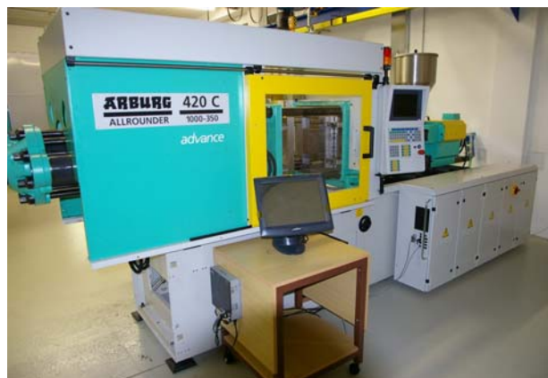
Figure 1. Injection molding machine Arburg 420C Allrounder with Workstation MPX
