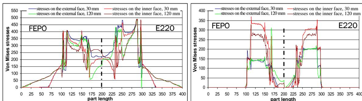
Figure 5. Equivalent stress distribution along the faces of the part before and after springback
