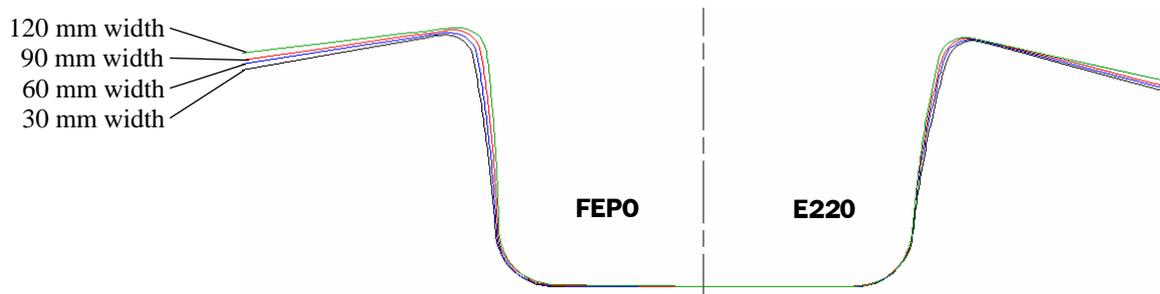
Figure 6. Sample width influence on springback of tailor welded stripes
