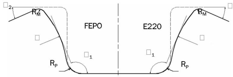
Figure 3. Geometrical springback parameters
