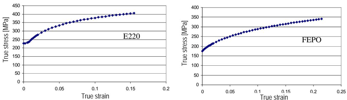
Figure 1. True stress-strain curves E220 and FEPO materials
