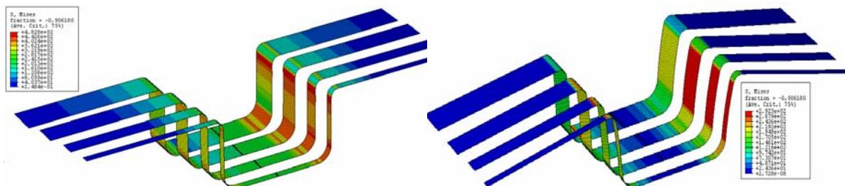
Figure 4. Equivalent stress before and after springback
