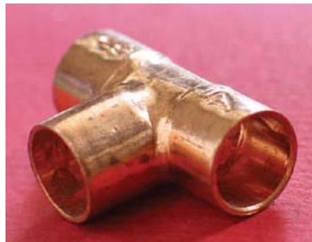
Figure 5. T- piece gotten by hydro forming [9]
