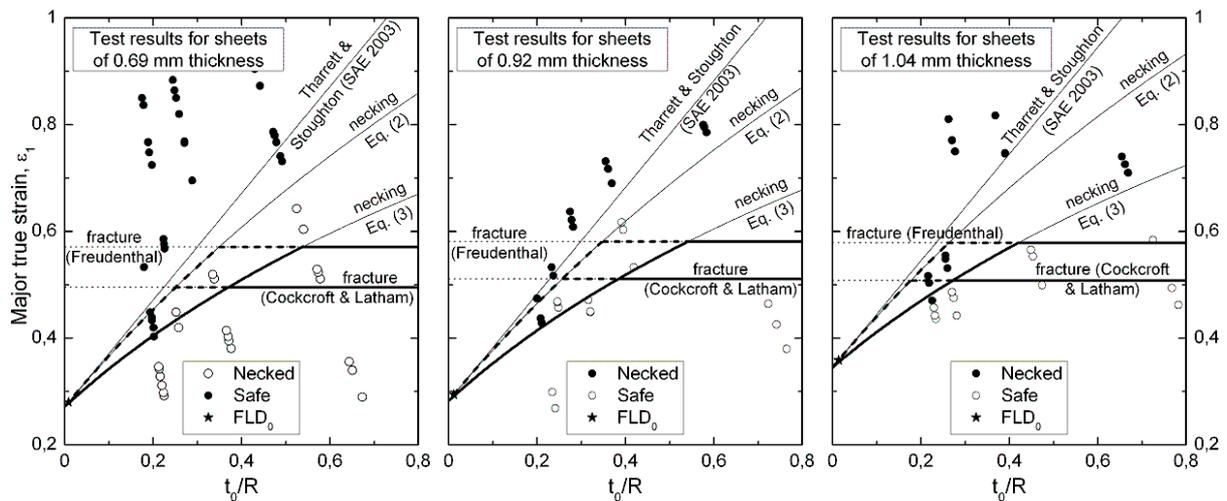
Figure 2. Major true strain on the convex (outer) side versus  $t_0/R$  ratio for 1008 AK steel sheets (Tharrett & Stoughton [1]). Theoretical Necking criteria and Fracture criteria are also plotted.
