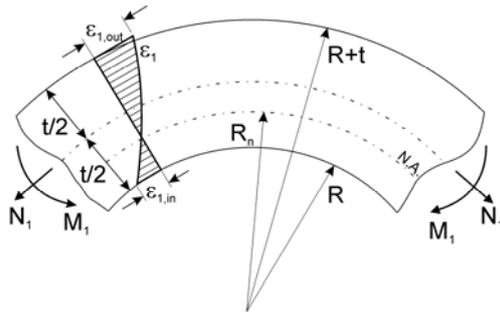
Figure 1. Variables in the stretch-bending.
