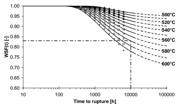
Figure 6. WSF(t) course in dependence on time and temperature of exposition for material P23
