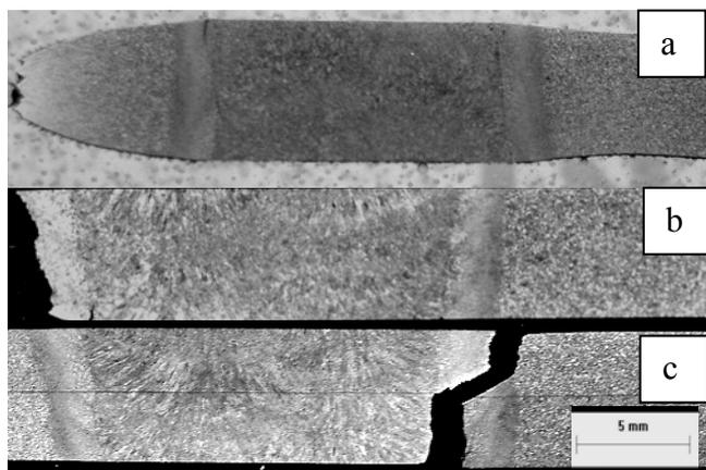
Figure 7. Damage type after creep tests
