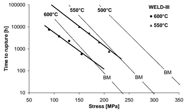
Figure 5. Creep strength of weldment - WELD III
