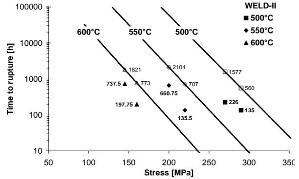
Figure 4. Creep strength of weldment - WELD II
