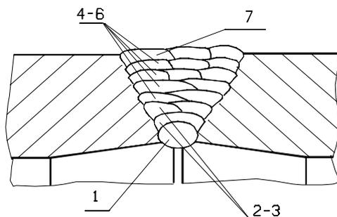
Figure 2. Order of welding metal layers
