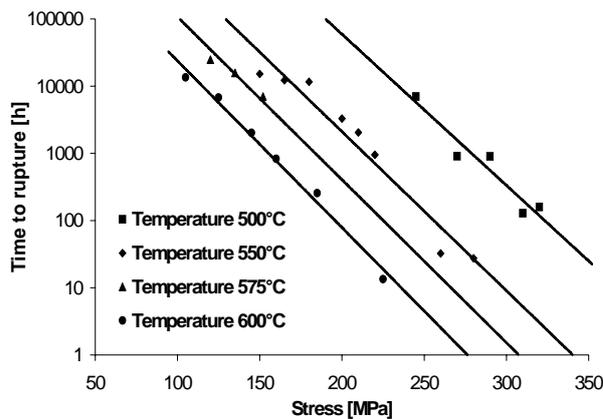
Figure 1. Creep strength evaluation of P23
