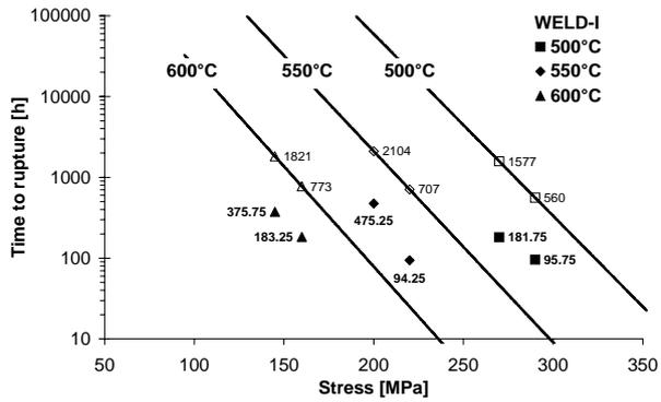
Figure 3. Creep strength of weldment – WELD I
